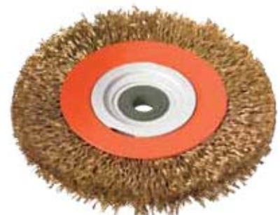
CCA – High Performance Wheel Traditional individual crimped wires (monofilaments) are substituted by crimped cables made of several wires each, resulting in 50% longer life than standard crimped wire.
